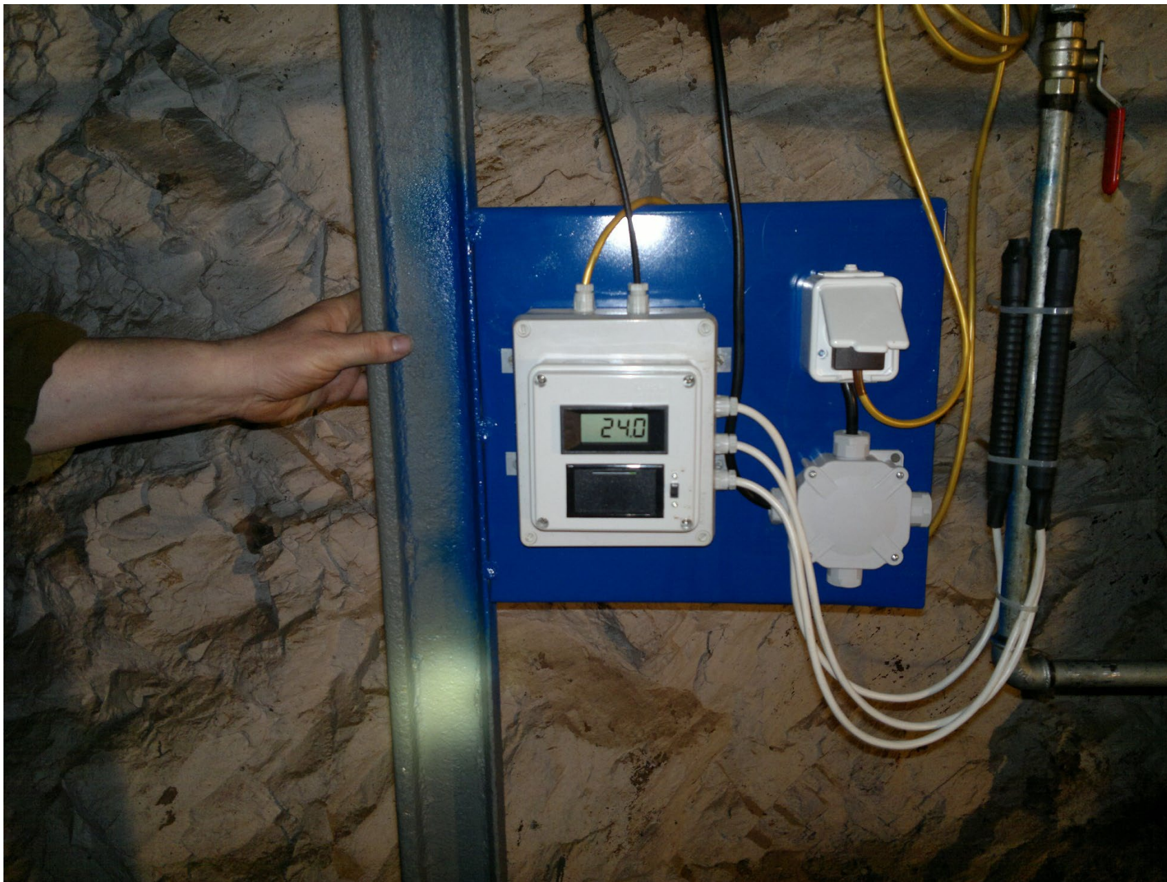
Fig. 4S. Measuring equipment directly in the mine while taking water from the spring (measured in kBq/L; photographed by the author T.Ř.).
