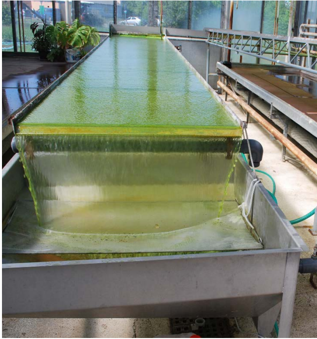
Supplementary Figure S1. Pilot-plant cultivation unit (a platform in a greenhouse) with Bracteacoccus bullatus CCA 1120, area 12 m 2 , volume 150 L, height of the suspension layer is about 10 mm.
